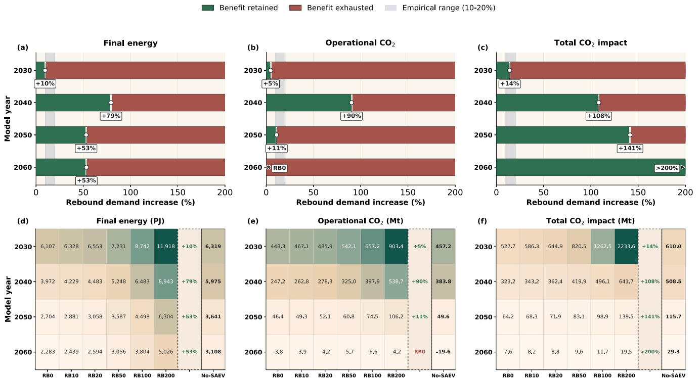
Fig. 10. CN60 rebound stress-test summary for High-NAEV relative to CN60-No. Top row: breakeven thresholds for (a) LDV final energy, (b) operational CO 2 , and (c) total passenger-LDV-related CO 2 in 2030, 2040, 2050, and 2060. Green indicates retained benefits, red indicates exhausted benefits, and markers denote interpolated breakeven thresholds. RB0–RB200 denote additional induced-demand increments of 0–200%, and the gray band marks the empirically informed 10–20% range. Bottom row: corresponding metric values for selected rebound cases together with the CN60-No benchmark.
